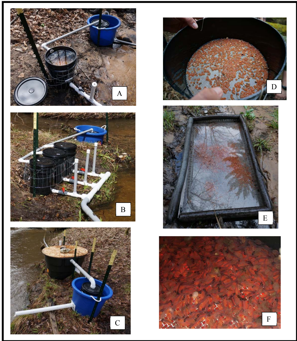
Figure 1. Pictures representing (A) a single-tank remote site incubator (RSI) at Hinton Creek, (B) a triple-tank RSI at Hinton Creek, and (C) stock-tank RSI at Peterson Creek used for rearing of Rainbow Trout eggs; egg trays (with Rainbow Trout eggs) used in (D) single-tank and triple-tank RSIs and (E) the stock-tank RSI; and (F) recently hatched Rainbow Trout fry on an egg tray.
