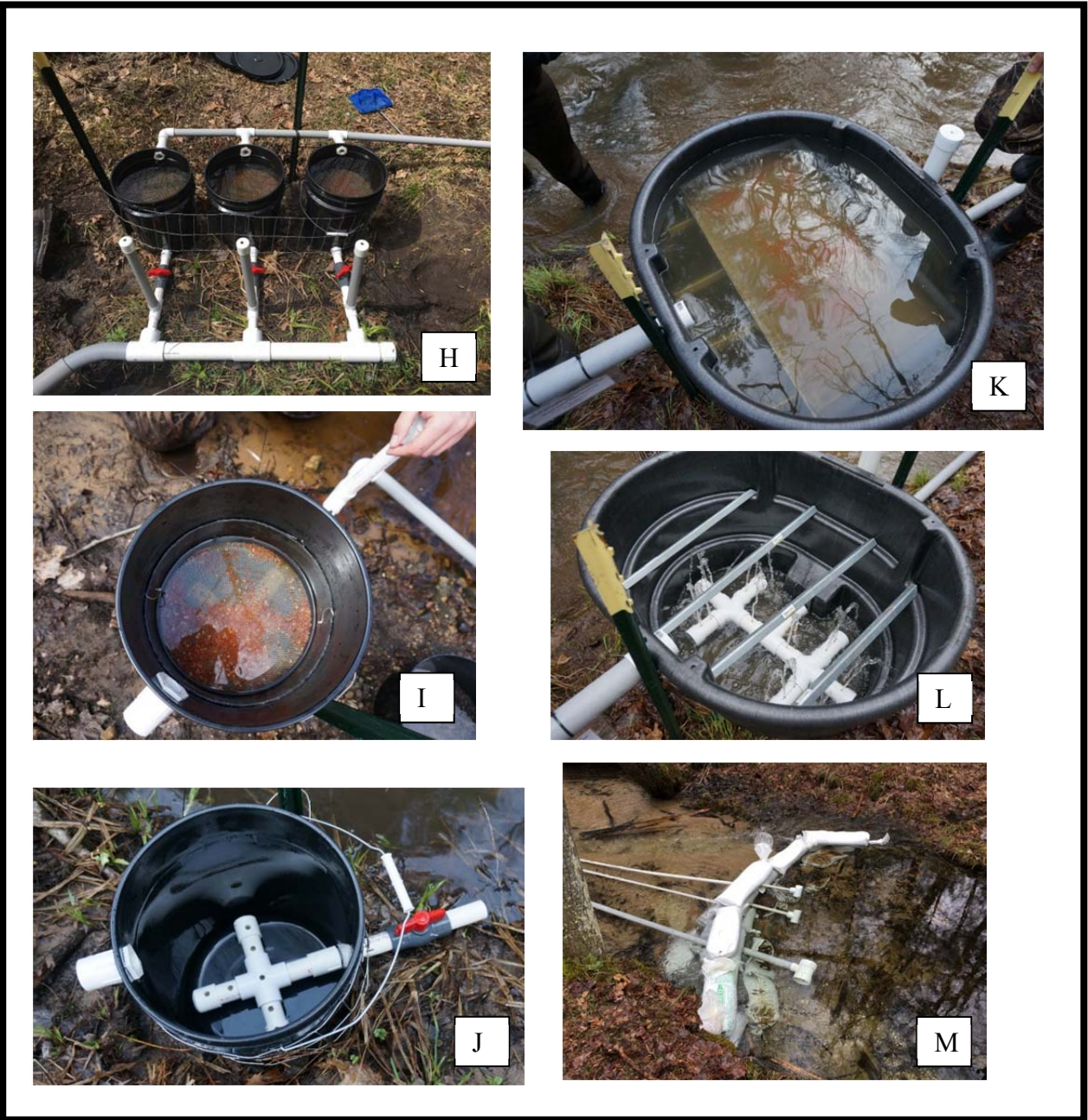
Figure B1 (cont.). (H) Triple-tank RSI with egg trays at Hinton Creek. (I) Single-tank RSI with egg tray in Hinton Creek. (J) Single-tank RSI with egg tray removed to show “+” shaped diffuser made from 1” PVC pipe and fittings with 3/8” holes. Stock-tank RSI with (K) rectangular egg tray present and (L) with the egg tray removed to highlight diffuser made from 2” PVC pipe and fittings with 3/8” holes. (M) An impoundment was required at Cedar Creek in order to increase the difference in elevation between the end of the water intake and the RSI to establish sufficient flow.
