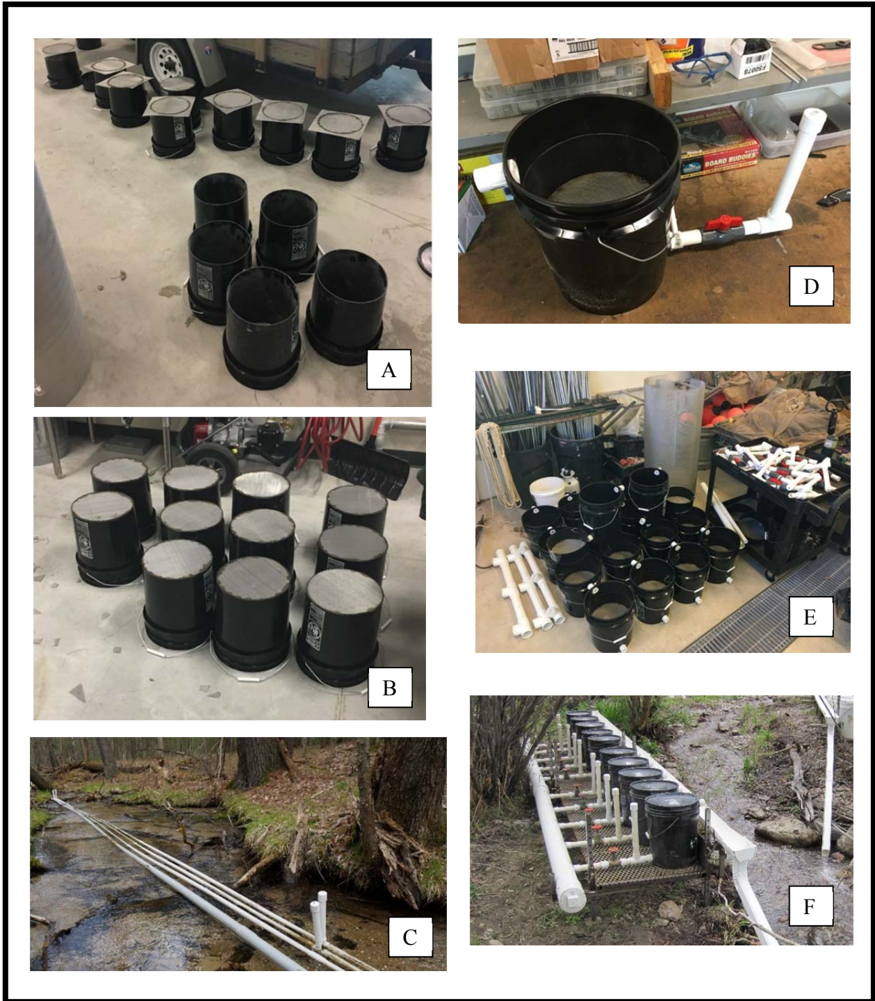
Figure B1. Construction of egg trays: (A) 5-gallon buckets with bottom cut off (foreground) and buckets with stainless steel mesh melted on the bottom prior to trimming excess mesh (background), and (B) 5-gallon buckets with the stainless steel mesh trimmed around the edges; the final step (not shown) is to cut-off top bucket (about 4-5" above mesh bottom). (C) Stand pipes (lower right corner) in 1" diameter water intake line at Cedar Creek were used to remove air from the line; note that 2" diameter water intake line for triple-tank remote site incubators (RSIs) is shown on left. (D) A completed 5-gallon bucket RSI with egg train installed and standpipe on water intake line. (E) All hardware for single-tank and triple-tank RSIs, including RSI "tanks" with eggs trays (center), PVC manifold for triple-tank RSIs (left), and standpipes for each RSI (right). (F) RSIs in-parallel in Montana illustrating the use of a "table" that could be used for triple-tank RSIs (MFWP 2013).
